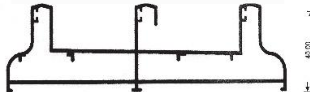
Triple track frame V 170-01
